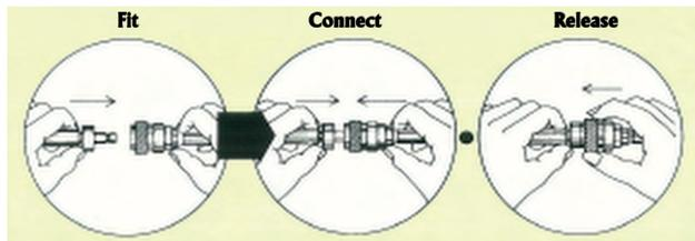
The Sentinel Safety-Z releases the connector using a unique reverse disconnect. This safety feature helps to prevent accidentally release of the coupler.
